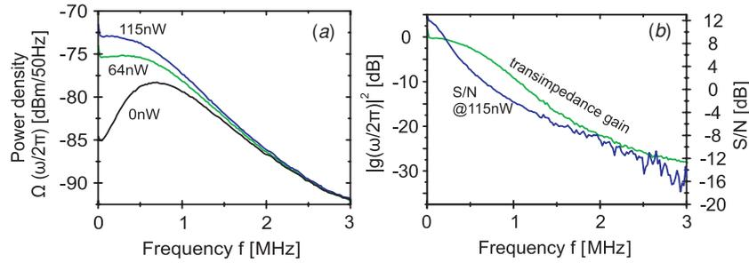
**Figure 4.** (a) Power spectrum of the detector when different, balanced dc light power levels are applied to the detector. (b) Frequency response of the detector, calculated from the raw data trace in (a) at 115 nW dc light power level. The gain drops by 3 dB within  $\sim 600$  kHz, which corresponds well to a shaping time of  $\sim 1.5 \mu\text{s}$ .
