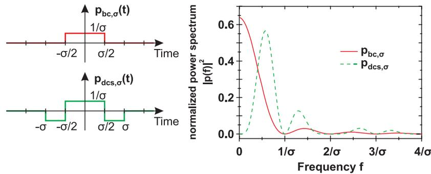
**Figure 5.** Integration pulse shapes  $p_{bc,\sigma}(t)$  and  $p_{dcs,\sigma}(t)$  and their power spectra  $|p_{bc,\sigma}(\omega/2\pi)|^2$  and  $|p_{dcs,\sigma}(\omega/2\pi)|^2$ . The integrated power spectra have been normalized to unity on the interval  $[0, \infty]$ .
