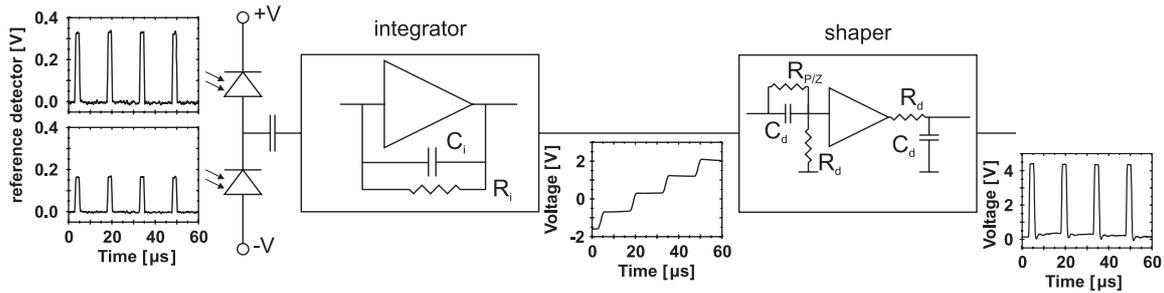
**Figure 1.** Schematics of the detector electronics. When an imbalanced signal is applied to the directly subtracted photodiodes as shown on the left, the differential photoelectrons are integrated. The time constant of the differentiator is adjusted such that it matches the decay time of the integrator. In consequence, the signal is zero between the pulses and the integral of the output pulses after the shaper is proportional to the differential photoelectrons.
