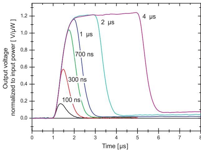
**Figure 2.** Output signal samples for different input pulse durations. The output signal has been normalized to the power of the input beam. The duration of the electronic output signal is extended by twice the shaping time. For long pulses, i.e. high photon numbers per pulse, a clear pulling of the detector baseline can be observed as an output signal which does not coincide with the level prior to the pulse.
