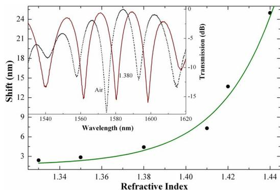
Fig. 4. (Color online) Shift of the interference pattern as a function of the external refractive index observed in a device with  $L=32$  mm. The solid circles are experimental data, and the continuous curve is a fitting to the data.  $\text{Shift}(\text{nm})=2.05046+B[\exp(RI/0.02503)]$  shows the expression that fits to the experimental points with  $B=2.3650 \times 10^{-24}$ . Inset, transmission spectra of the device in air and in liquid with an index of 1.380.
