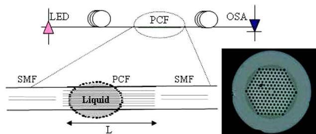
Fig. 1. (Color online) Schematic of the experimental setup, micrograph of the PCF used, and drawing of the interferometer. SMF, single-mode fiber; LED, light-emitting diode; OSA, optical spectrum analyzer; L, length of PCF.
