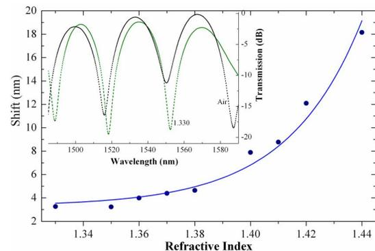
Fig. 3. (Color online) Shift of the interference pattern as a function of the external refractive index observed in a device with  $L=17$  mm. The solid circles are experimental data, and the continuous curve is a fitting to the data.  $\text{Shift}(\text{nm}) = 3.29163 + A[\exp(RI/0.02659)]$  shows the expression that fits to the experimental points with  $A = 4.75282 \times 10^{-23}$ . Inset, transmission spectra of the device in air and water.
