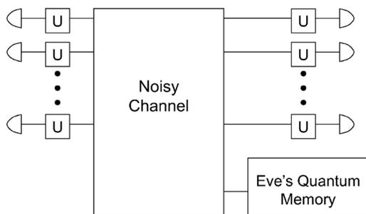
FIG. 2. A tripartite pure state is prepared by Eve, who send two of the particles to Alice and Bob and keeps one. From the Alice and Bob viewpoint the situation resembles a standard noisy channel. The honest parties perform measurements at the single copy level, possibly with some preliminary filtering step. Eve keeps her quantum states and can arbitrarily delay her collective measurement.
