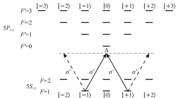
Figure 1: Levels and transitions relevant for spin squeezing on the D<sub>2</sub> line in  $^{87}\text{Rb}$ .
