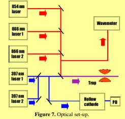
Figure 7. Optical set-up.
